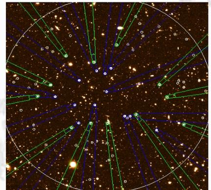
Fig. 7: I-band image of the FORS Deep Field with KMOS pickoff arms assigned to 24 Extremely Red Objects. The blue arms belong to the lower plane (and can therefore be vignetted by arms in the upper plane) whilst the green arms patrol the upper plane. The positioning efficiency of the arms has been checked against a number of important science cases which demonstrate a high multiplexing factor on interesting targets.
