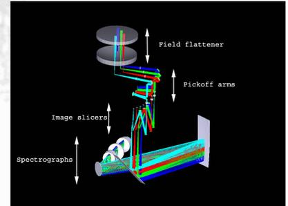
Fig. 3: Optical raytrace through four pickoff arms, their associated IFUs and one of the spectrometers. Light exiting the pickoff arms is brought to an intermediate focus using a 3-element K-mirror, which aligns the edges of all 24 IFU fields on the sky so that they can be put into a compact sparse array configuration for blind surveys of contiguous areas on the sky.
