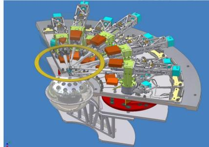
Fig. 2: One of the three integrated pickoff and IFU sub-modules showing the tiered mounting plates for the pickoff arms, the filter wheels and the IFU optics. Each sub-module is attached to the main cryogenic optical bench within the cryostat. At the centre of the unit is shown the integrating sphere of the calibration unit and the ring mirror which reflects light from the calibration sources into the pickoff arms.
