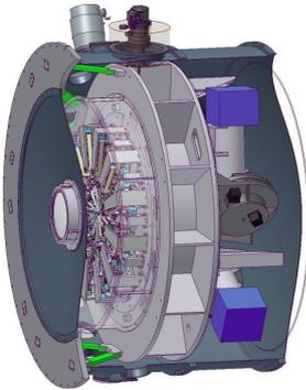
Fig. 1: Cutaway view of the main KMOS cryostat showing the entrance window and the pickoff arm module at the front, and the spectrograph module at the rear. The cryostat is an aluminium/stainless steel hybrid to reduce weight. Not shown here are the electronic racks which are mounted on a corotating frame behind the cryostat.
