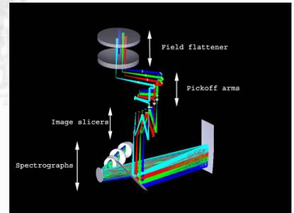
Fig. 3: Optical raytrace through four pickoff arms, their associated IFUs and one of the spectrometers. Light exiting the pickoff arms is brought to an intermediate focus using a 3-element K-mirror, which aligns the edges of all 24 IFU fields on the sky so that they can be put into a compact sparse array configuration for blind surveys of contiguous areas on the sky.
