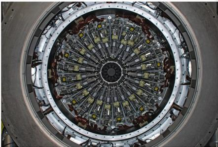
Fig. 4: Front view of the KMOS cryostat showing the 24 robotic pickoff arms surrounding the patrol field. The cryostat diameter is approximately 2 metres. The arms patrol in one of two different planes to reduce interference.
