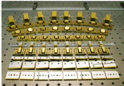
Fig. 6: Gold-coated diamond machined optics for one of the three 8-IFU modules in KMOS. The total image slicer system for all 24 channels contains 1152 optical surfaces with form errors in the range 10-15nm and surface roughness  $< 10$ nm.
