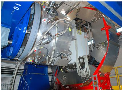
Fig. 5: Completed KMOS cryostat under test on the flexure rig at the ATC in Edinburgh. The red structure behind the cryostat is the CACOR unit which corotates with the spectrograph and contains all the control and housekeeping electronics.
