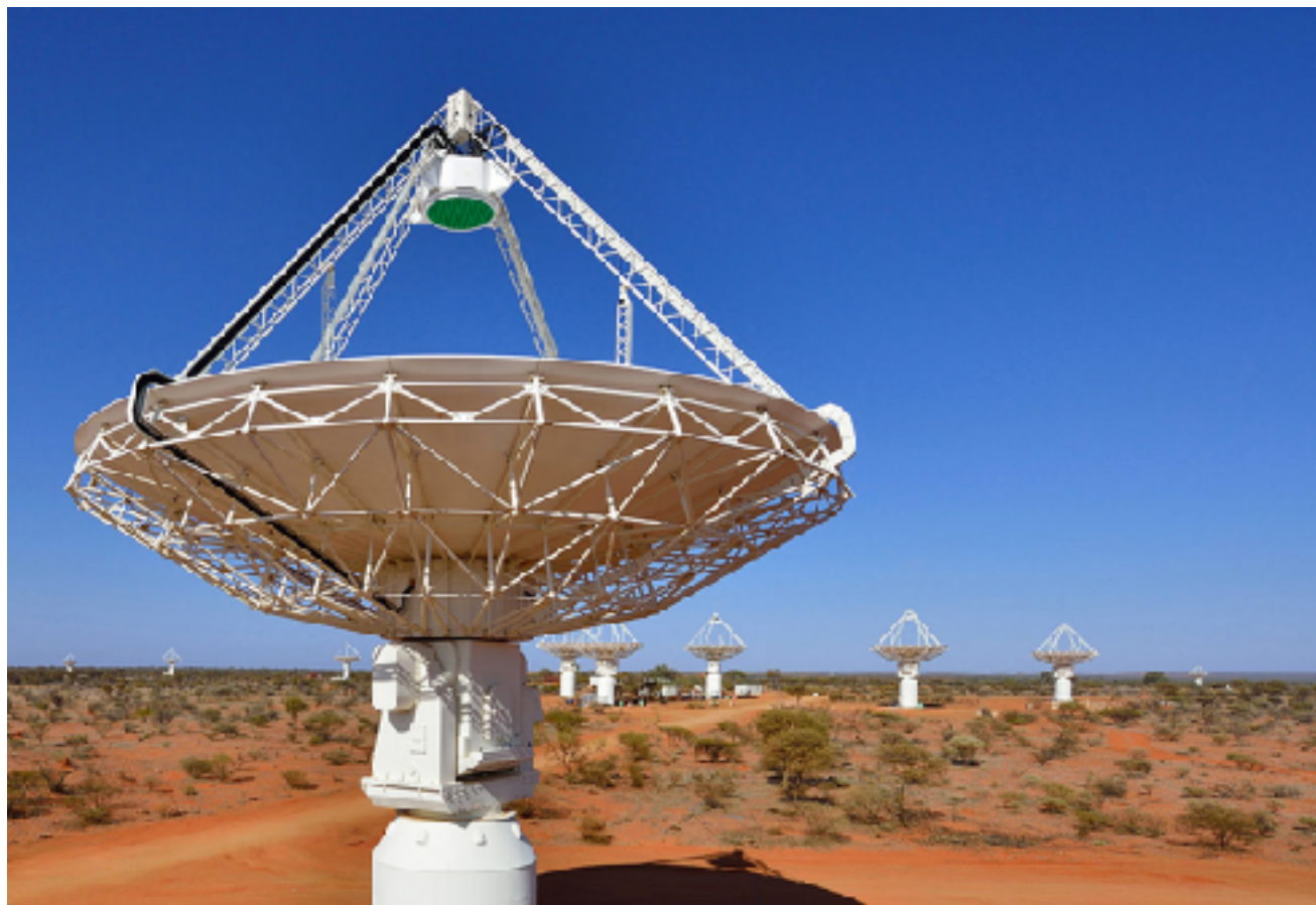
ASKAP: Phased-array feed
