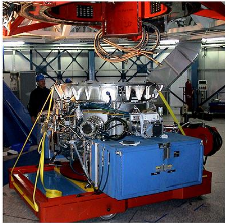
VISIR under the Cassegrain Focus of the 8.2-m VLT Melipal Telescope
