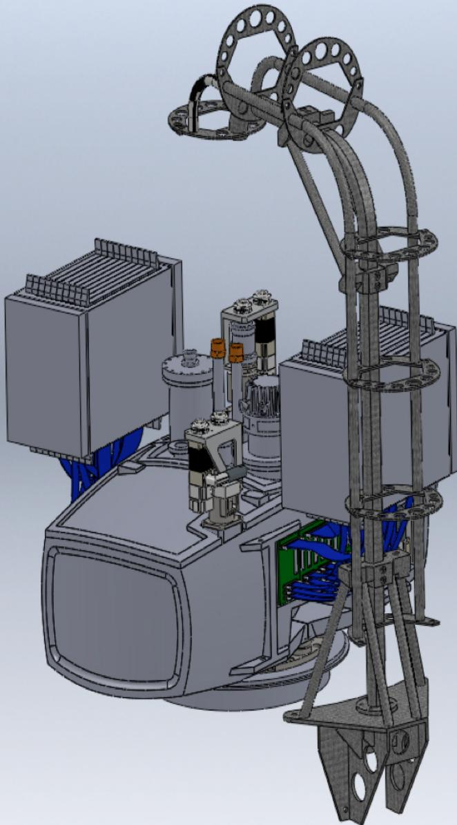
Body of camera made of carbon fiber, shaped to minimize wall thickness
