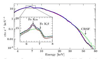
FIG. 10.— Spectrum with 15 ks exposure of Vela X-1 taken by NuSTAR. The red curve shows focal plane module A and the blue curve is from B. The inset shows the Fe-line region. The good broad band response enables NuSTAR to measure both Fe-line fluxes and high energy continuum. A Cyclotron Resonance Scattering Feature (CRSF) is seen with high significance at 55 keV.
