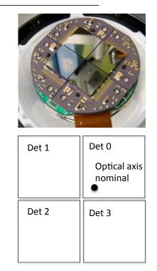
FIG. 5.— Photo of a *NuSTAR* focal plane (top). The focal plane consists of a  $2 \times 2$  array of CdZnTe pixel detectors, each with  $32 \times 32$  pixels 0.6 mm in size. The detectors are referred to as Det 0-3. The optical axis nominal location is approximately 1' from the chip gaps on Det 0 (bottom).
