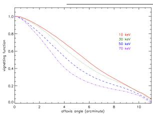
FIG. 4.— The reduction in effective area as a function of off-axis angle resulting from vignetting in the optics. The curves show the vignetting function for different incident energies. Due to the tightly nested low-graze-angle design and the change in reflectance of the shells as a function of energy, the vignetting is strongly energy dependent above 15 keV.
