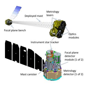
FIG. 1.— Diagram of the observatory in the stowed (bottom) and deployed (top) configurations.
