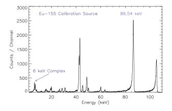
FIG. 9.— Spectrum of the <sup>1</sup>55Eu flight calibration source for focal plane module A taken during on-orbit commissioning. At energies below 50 keV the resolution is 400 eV FWHM and is constant with energy, being determined by the electronic noise. Above this the energy resolution broadens due to charge trapping effects in the detector, reaching 1.0 keV FWHM at 86 keV.
