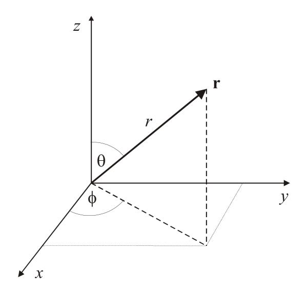
Differential volume element in spherical polar coordinates.
