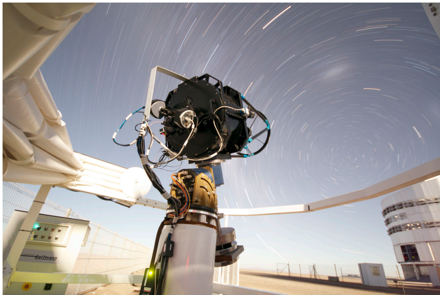
The CfAI 0.5 metre turbulence monitoring telescope at Cerro Paranal, Chile, home of the ESO Very Large Telescope (VLT) and nearby 40 metre European Extremely Large Telescope (ELT). Photo: tim Butterley.
