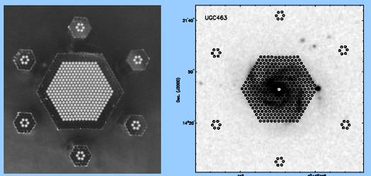
**PPak:** Left: The fiber-based PPAk IFU, developed for the DiskMass Survey (Verheijen et al. 2004), has a large field of view, with 331 science fibers and 36 sky fibers. Right: The PPAk fiber-footprint overlaid on top of UGC 463, one of the galaxies in our sample.
