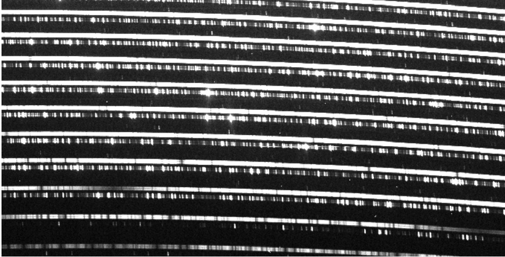
Figure 20: Region within a raw image of a spectrum of the star HIP66974 and a calibration lamp, taken with ESO’s FEROS spectrograph in June 2015 (Data set SAF+FEROS.2015-06-13T23:16:46.772). Retrieved from ESO’s Science Archive on 24 April 2019
